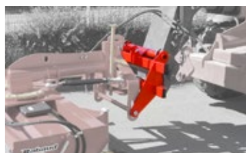
Mixed hitch for second carrier like a telescopic
