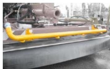
High pressure watering line, 4 sprayers
